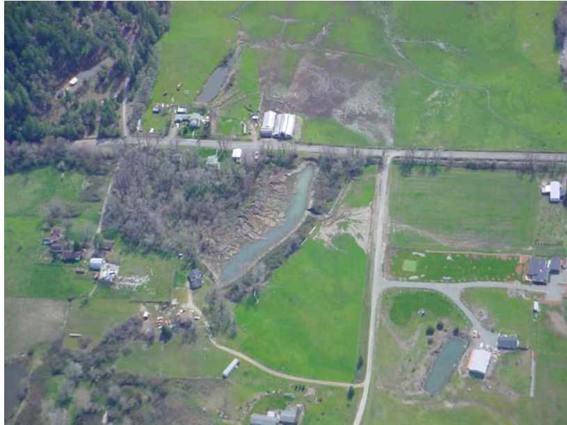
Fig: 58 Aerial photo showing pond on Panther Gulch where dam failure resulted in mudflows and flooding of lower Williams Valley
